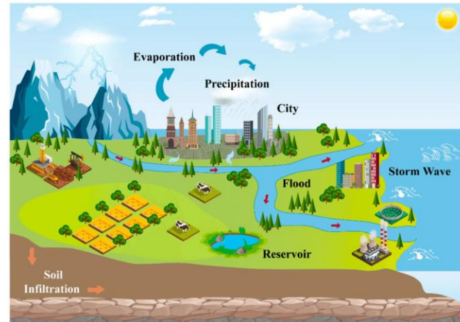
The impact of urbanization on the hydrological cycle: increased runoff and decreased infiltration.
